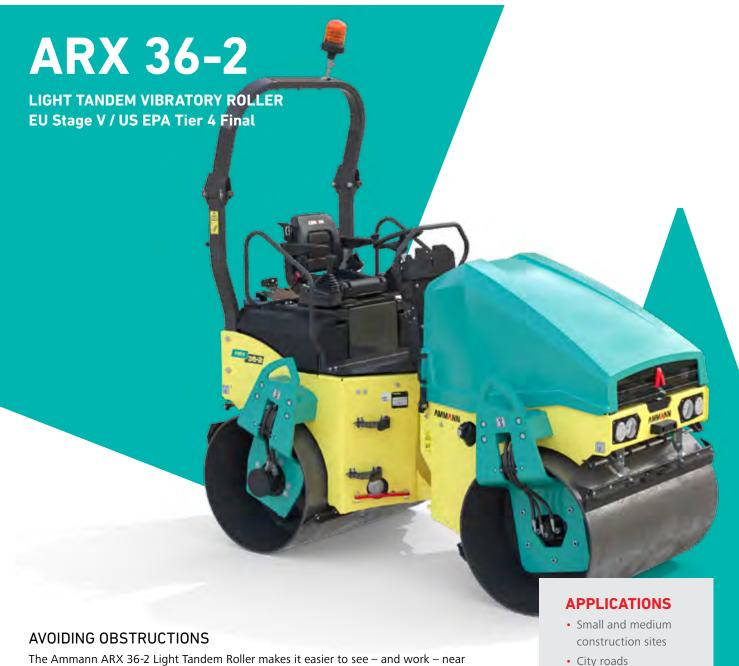
The Ammann ARX 36-2 Light Tandem Roller makes it easier to see – and work – near obstructions. The roller features a new articulating joint that enables quick drum adjustment from in-line to offset configurations, helpful when working close to obstructions. Operators need watch only one drum, knowing the second will be a safe distance from the obstacle. The in-line drum setting is available when it's time for productivity in open spaces.
