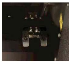
The control of your loader is as easy as it gets. One pedal for forward direction and one for reverse.
