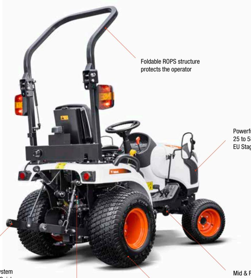
Foldable ROPS structure protects the operator
