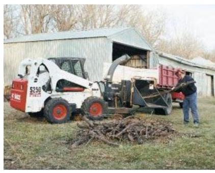
Bobcat Remote Attachment Control (RAC) system - This system allows the operator to start or stop the loader's engine and chipper rotation when standing beside the attachment.
